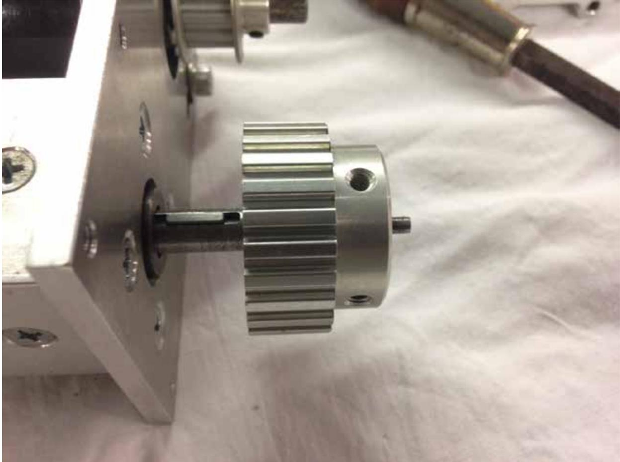
5. Replace the 5/16-24 Nylock nut that was removed in step 3. Torque till snug or 35 inch pounds holding the pulley to keep the lead screw shaft from rotating.
