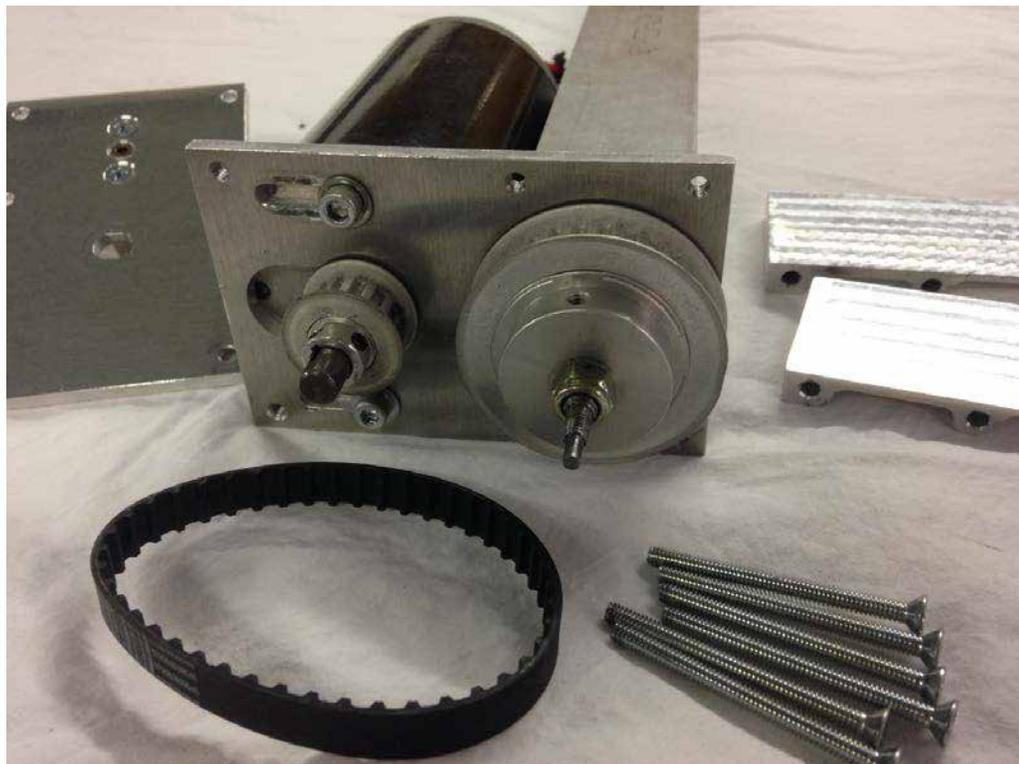
3. Remove the 5/16-24 Nylock nut securing the driven 30 tooth pulley to the lead screw. Using 2 flat blade screw drivers, carefully pry the pulley off the lead screw shaft as shown. Be careful not to lose the 2mmx10mm machine key captured between the pulley and shaft. Do not remove the race spacer located under the pulley, this will support the new pulley as it did the original.
