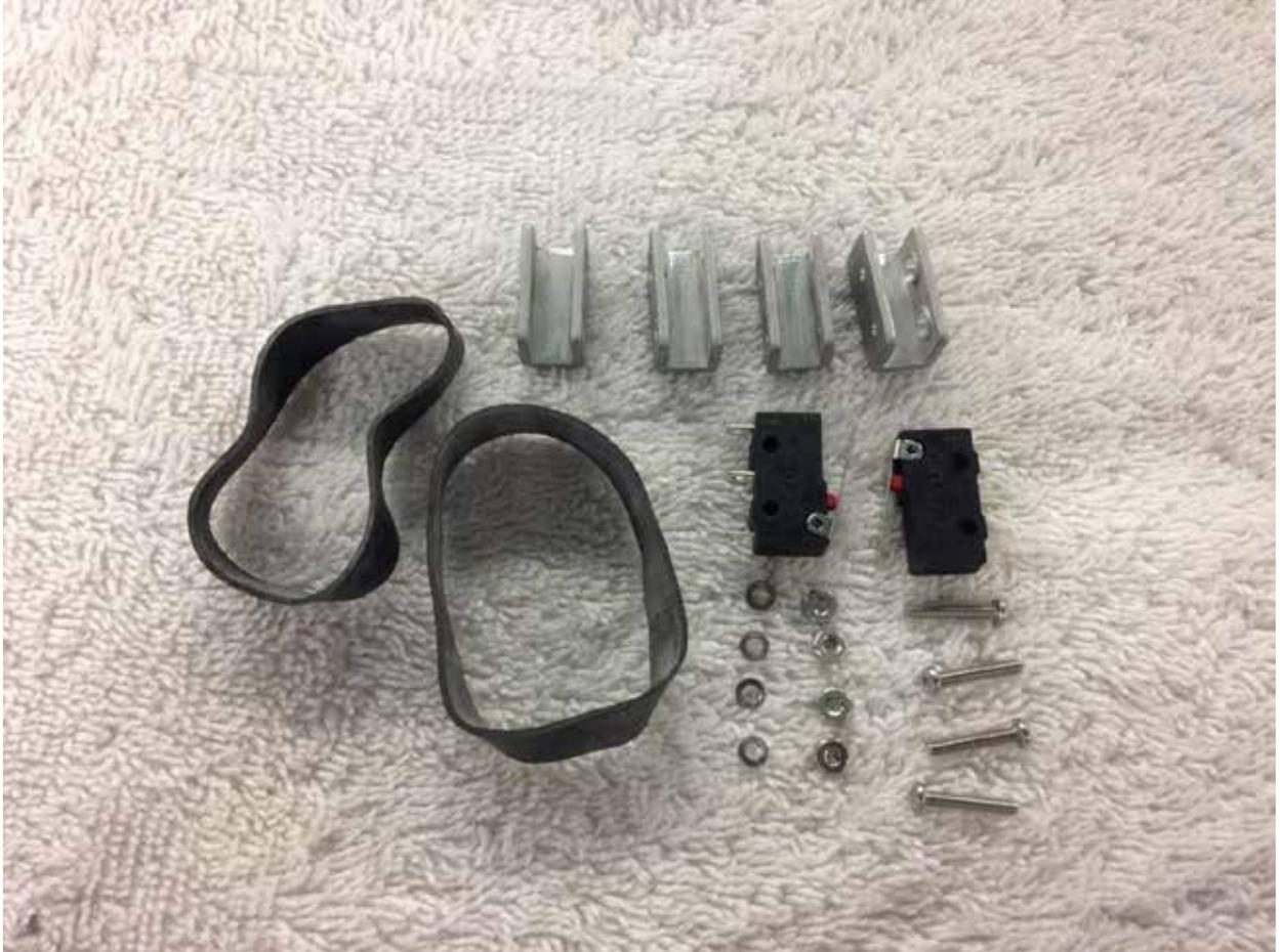
1. Assemble both limit switch assemblies as pictured in Fig. C. Each one of these two assemblies should include one limit switch, two limit switch brackets, two 2-56 x .500 philips machine screws, two #2 lock washers and two 2-56 hex nuts. Leave screws slightly loose.
